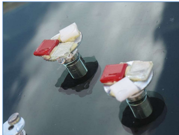
Image 3: Two coupons and steel washers were attached to the front windshield of the truck using an inside static magnet.
