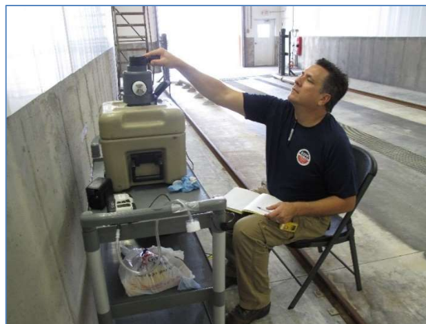
Image 5: Preparing the SKC air sampling instrument inside the automated power washing bay.
