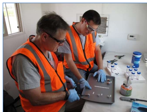
Image 4: Treated coupons are being prepared for labeling, storing, and transport to the Mesa laboratory for final assaying and enumeration of viable MS2 phages.
