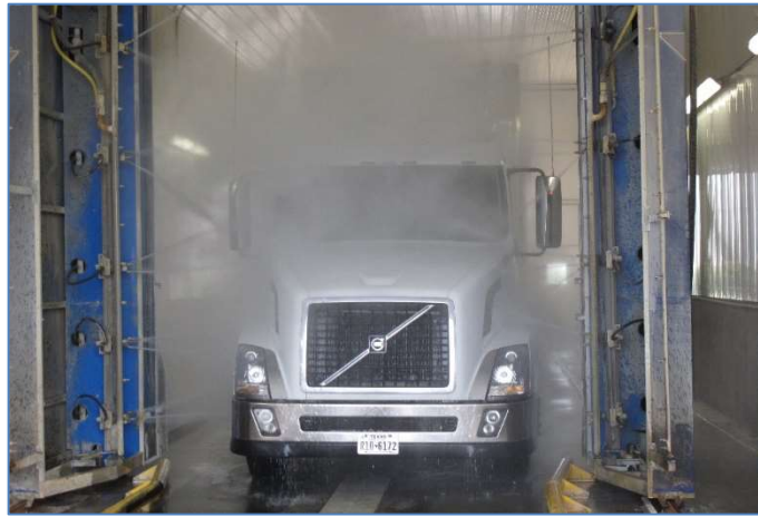
Image 1: Power washing a tractor-trailer with the Whitening power washing gantry system.
