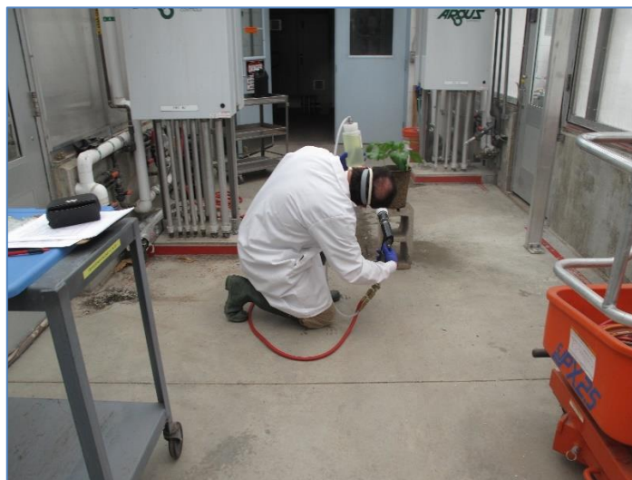
Figure 1: Chemical application to plant foliage using the ESS electrostatic sprayer.
