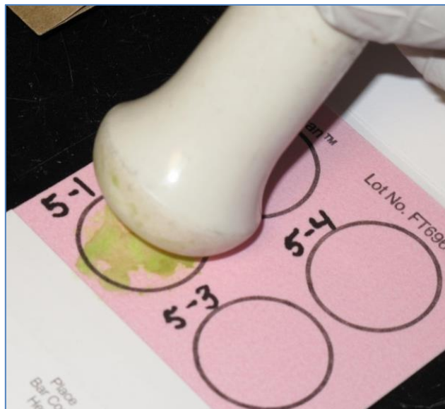
Figure 5: Applying leaf tissue paste from a mortar pestle to a labelled FTA card.
