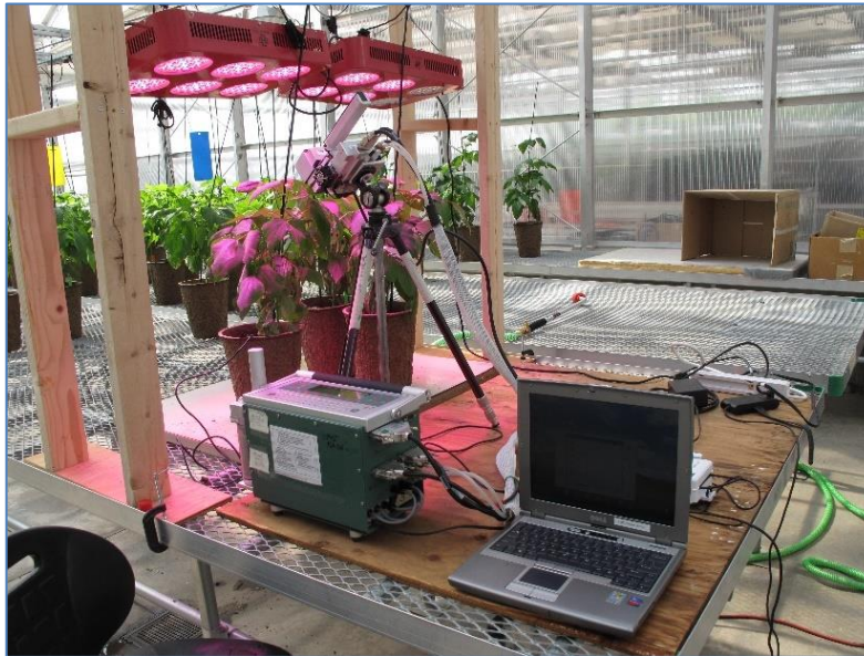
Figure 2: Measuring gas exchange of kidney bean foliage using the LICOR 6400 XT instrument and LED grow lamps to ensure uniform light conditions during measurements.
