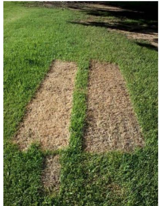
Figure 4: Patches of kikuyu grass treated with Slow-wave applicator connected to a 2.0 kW, 2.45 GHz microwave source – 2 minutes to treat approximately 2 m 2 (Note: this image was captured approximately 24 hours after treatment).
