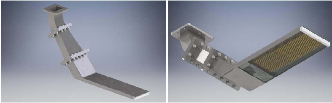
Figure 2: 3-D models of a comb type slow-wave applicator operating at 2.45 GHz (above) top view and (below) bottom view showing the comb.
