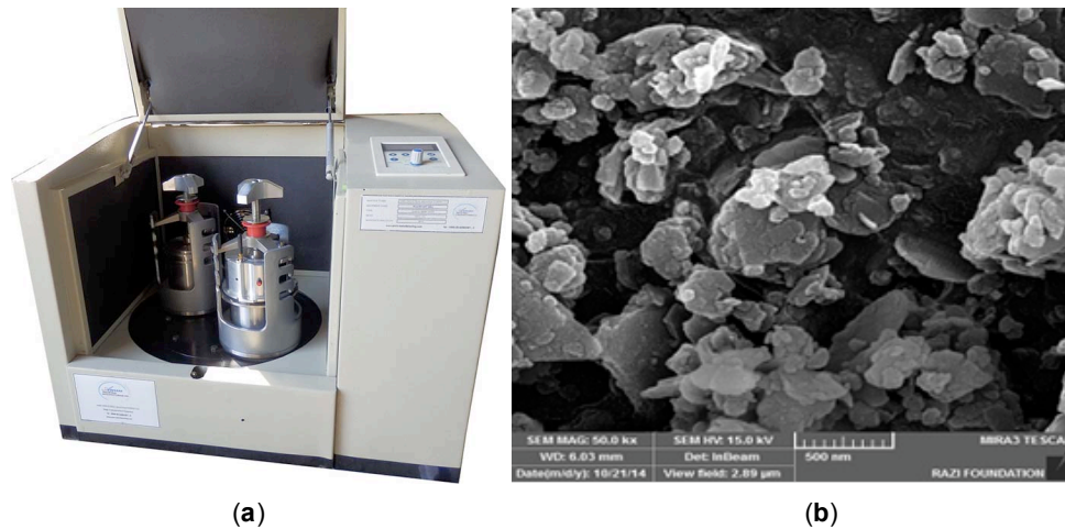
Figure 3 (a): A general view of ball-mill equipment. (b) An example of FESEM image of kaolinite.
