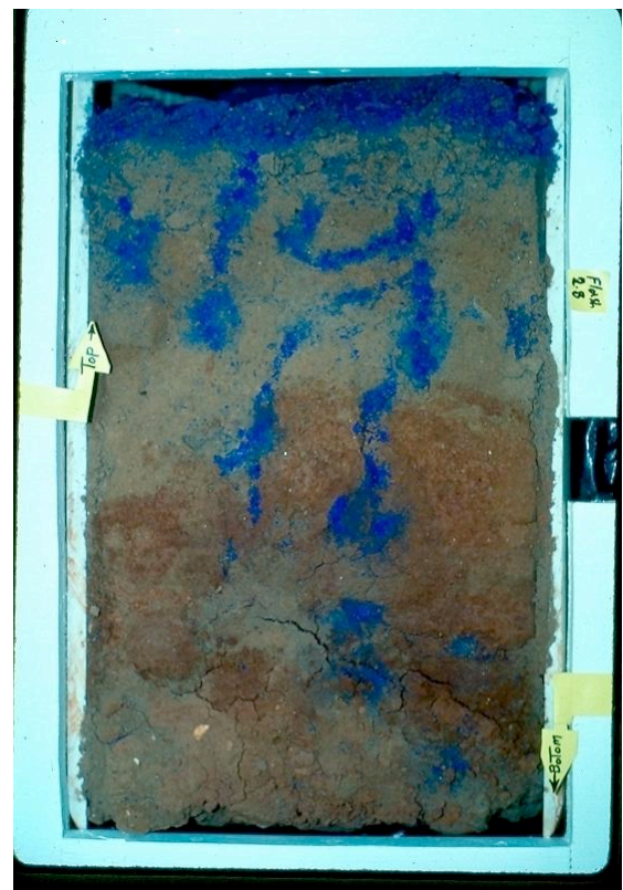
Figure 2: Dyed soil core showing substantial differences between stained versus unstained areas.
