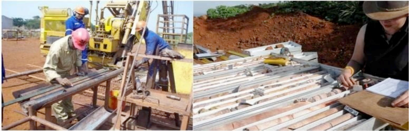
Figure 2: Geotechnical Drilling and Measurement of RQD from drill cores.
