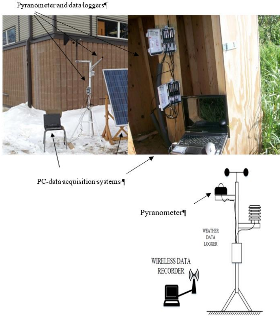
Figure 3: Photograph and schematic diagram showing the solar-logging station used for measuring the monthly average daily solar radiation received on a horizontal surface positioned on Lakehead University's campus nearby TBRHSC site for use as inputs into the mathematical predictive model.
