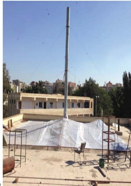
Figure 1: a. Schematic overview of the Solar Chimney principle. b. Picture of the system.
