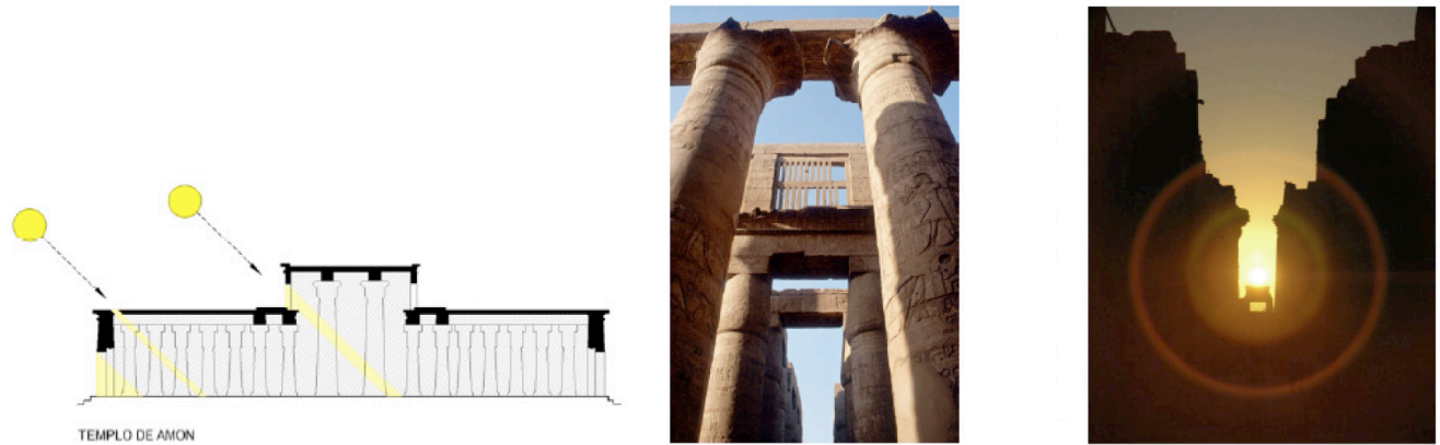
Figure 7: Left, and centre, the Temple of Amon at Karnak with detail of the zenith illumination in the hypostyle hall (source: author's interpretation). Right, sunrise at the winter solstice on the main axis of the temple of Karnak (Source: Belmonte, 2005).
