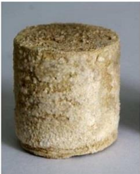
Figure 1: A sample of cement stone formed from the composition of alumina cement in combination with portlandcement and microsphere additives and fine-dispersed ash.
