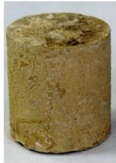
Figure 2: A sample of cement stone based on highly alumina cement combined with portlandcement, slag and barite additives.
