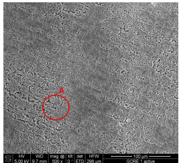
Figure 5: PTFE membrane surface at 500x magnification, highly porous region used in the analysis is circled and indicated as A.
