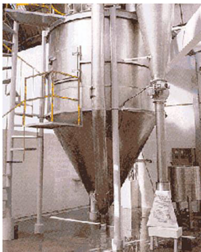
Figure 3: Spray dryer device [3].
